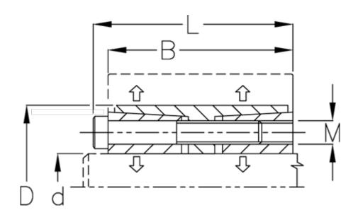
$\begin{array}{lll} \text{B mm} & = 45 \\ \text{d H8 mm} & = 28 \\ \text{D mm} & = 55 \\ \text{Fit tolerance} & = \text{Aksel h8, Nav H8} \\ \text{F kN torque} & = 70.0 \\ \text{L mm} & = 51 \\ \text{M mm} & = \text{M6} \\ \text{P N/mm2 surface pressure on shaft/hub} = 90 \end{array}$
